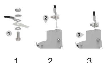
Mount the accessory in the wire or busbar (10Nm)
